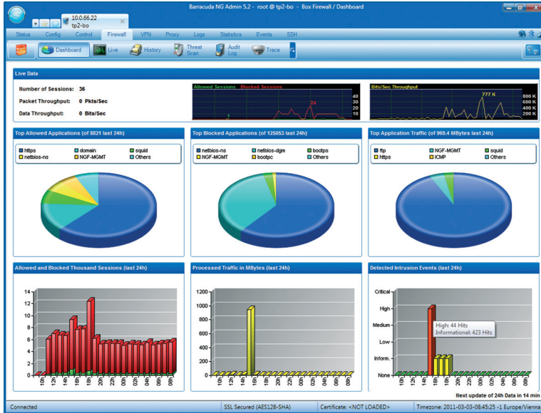
The dashboard displays a live view on a selection of important status and statistics data such as top application usage, detected intrusion events, number of active sessions, etc.
